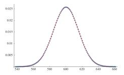
Bullets: pmf of  $S_{1000} \sim \text{Bin}(1000, 0.6)$ Red curve: pdf of  $X \sim \mathcal{N}(600, 240)$
