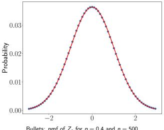
Bullets: pmf of  $Z_n$  for p = 0.4 and n = 500Red curve<sup>1</sup>:  $X \sim \mathcal{N}(0, 1)$
